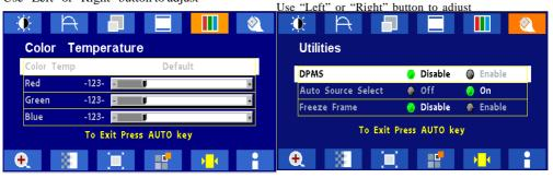
Push "Left" or "Right" to select Color Temp betweenPush "Up" or "Down" button to select between "Default", "System 1", "System 2", "System 3", or "DPMS", "Auto Source Select", or "Freeze Frame" "System 4" then push "Select" then push "Select" Use "Left" or "Right" button to If "System 1, 2, 3 or 4" were slected, push "Up" or "Down" button to select between "Red", "Green", or
